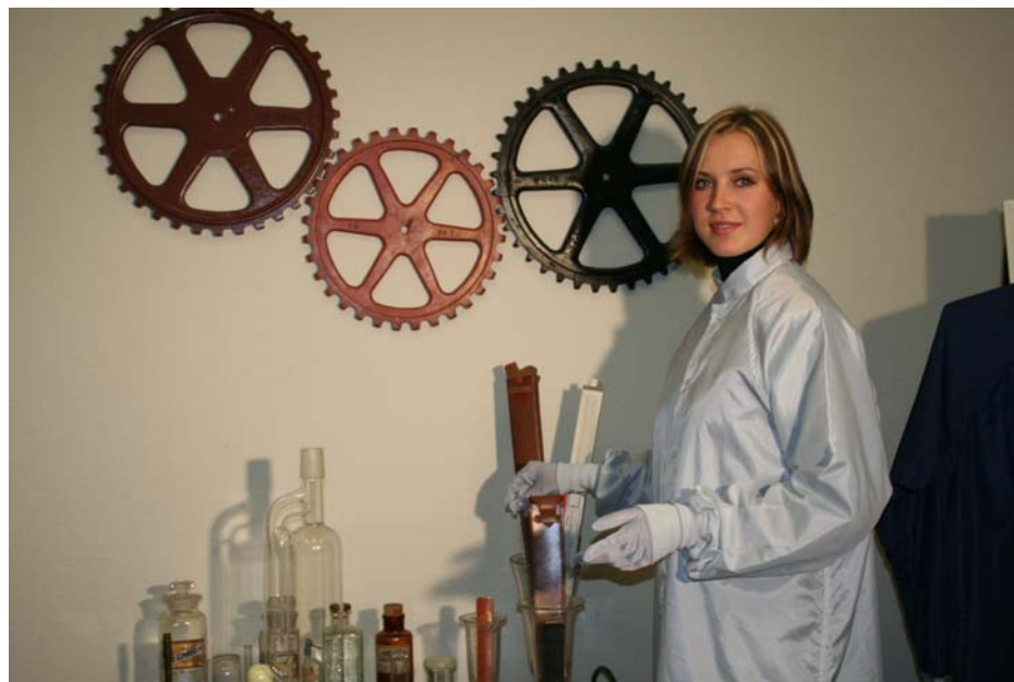
Fig. 13. Static dissipative lab coat and gloves coated with light-colored conducting polymer.
