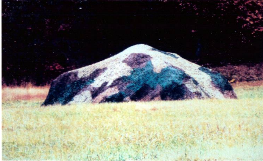
Fig. 9. Multispectral camouflage netting. In addition to providing the radar and IR camouflage, the conductive polymer-coated net functions as the main webbing of the overall camouflage netting.
